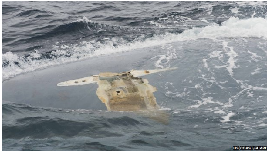
The US Coast Guard issued photographs of Cheeki Rafiki's upturned hull showing its keel had broken off
